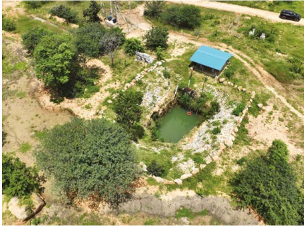
▲ Revived well, storing seasonal rainfall and distributing water to the entire site, with a total capacity of 550,000 L.
