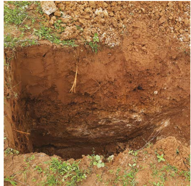
▲ Soil profiling at 10 ft to understand layers, depth and texture of soil
